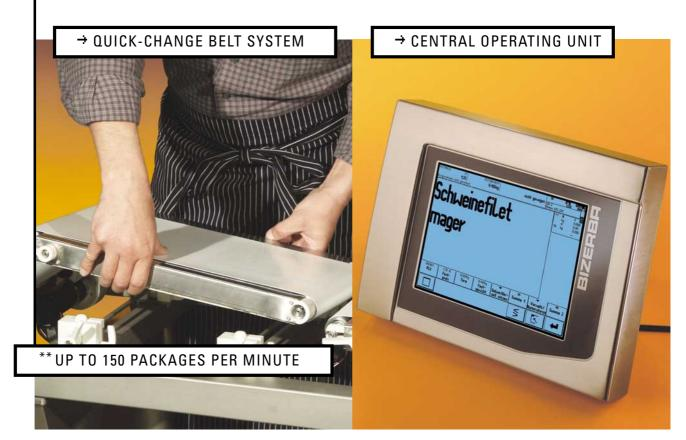
labeling rate of up to 150 packages per minute. The modular print engine of the GLMH labeler provides easy-to-change print-heads, easy cleaning and convenient insertion of paper and Thermal Transfer Film rolls.
